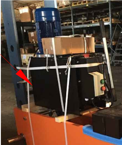
Fig. 10 Hydraulic Unit and mounting brackets as shipped from the factory
