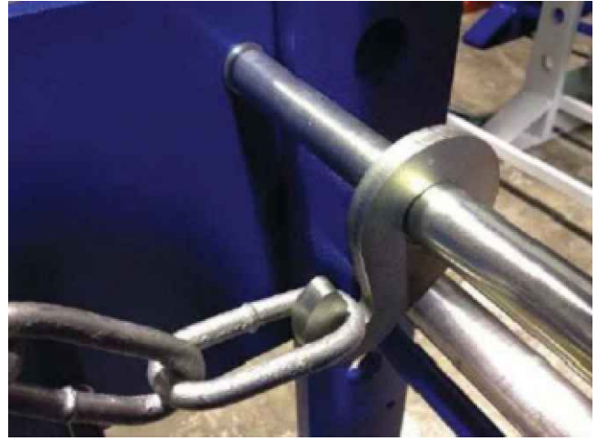
Fig. 23 Lifting chain on table hook
