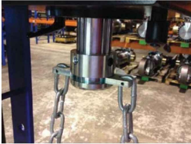
Fig. 22 Lifting chain bridge around piston head
