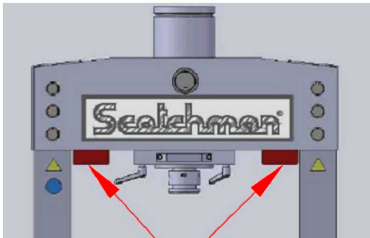
Fig. 8 Positioning Forks of Forklift Truck
