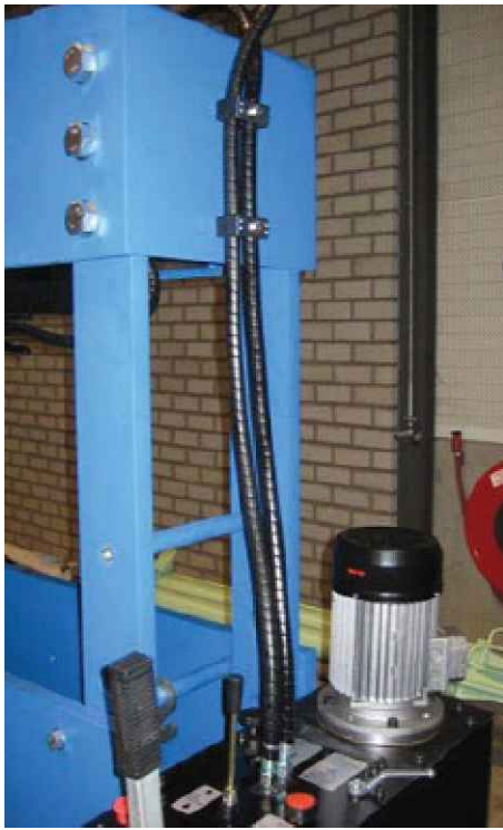
Fig. 11 Keep hoses straight - no sharp bends
