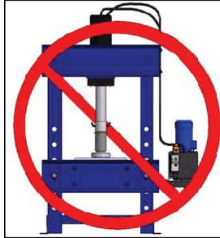
Fig. 5 Max. force with long stroke
