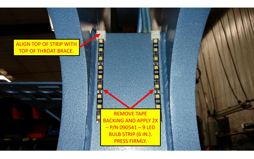
**NOTE:** THE 3M VHB TAPE IS A PRESSURE ACTIVATED ADHESIVE. IF **LIGHTLY APPLIED** TO A SURFACE, IT MAY BE POSSIBLE TO PULL OFF AND REAPPLY. IF **FIRMLY ATTACHED**, IT WILL BE NEAR IMPOSSIBLE TO MOVE.
