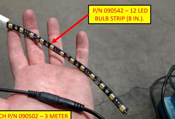
ATTACH P/N 090502 – 3 METER EXTENSION CORD TO STRIP.
