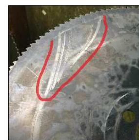
The material must be properly seated and solidly clamped in the vise. If the material moves during the cut it can bend or break the saw blade. Pick-Up can be a major contributor.
